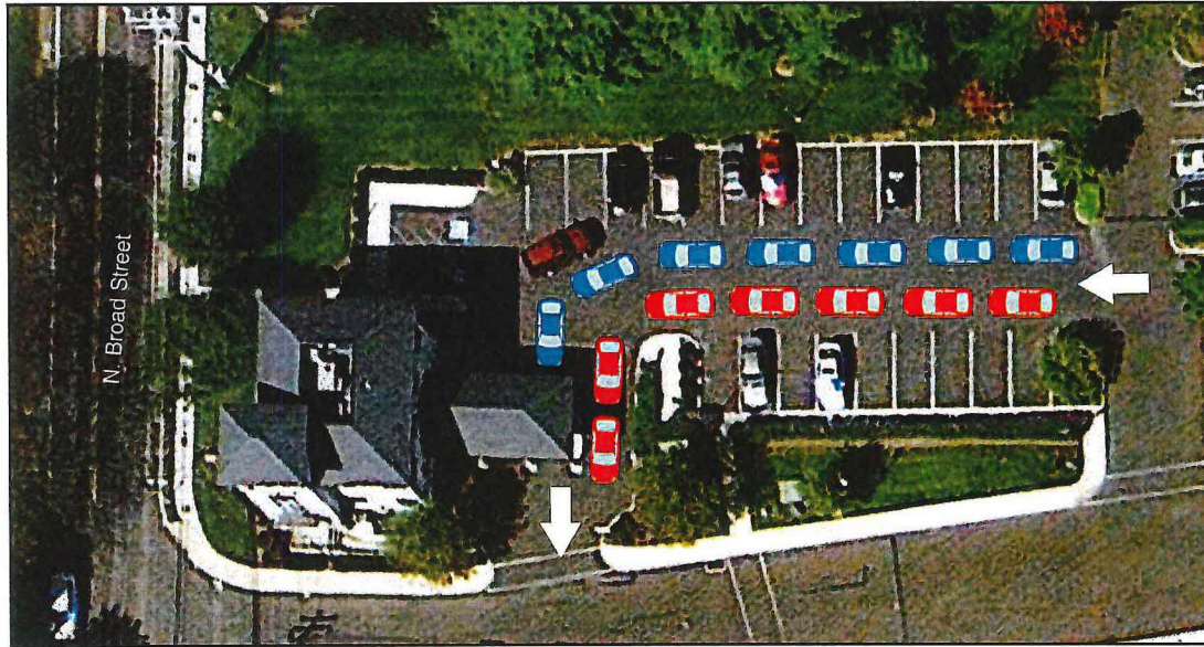
Traffic stacking at Drive-Through Facility located in the rear of the building
